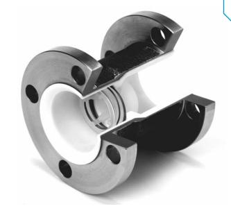
The **Check-All Flanged & Drilled** — **Fluoropolymer (PTFE) Lined (HT)** check valve is a one piece body with ANSI/ASME B16.5 Class 150 flanged ends. The valve has a solid one piece PTFE liner which covers the flange faces out to the raised face diameter. All wetted surfaces are fluoropolymer (PTFE/FEP/PFA) including the FEP encapsulated stainless steel spring.
