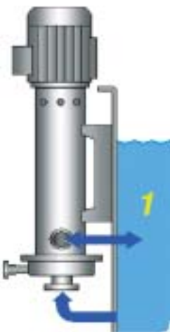
4. Version IMO , in which the pump is placed outside the vessel. A bypass connection (1) must be utilised as an overflow. On the picture you can also see an additional cleaning connection (2) (optional).
